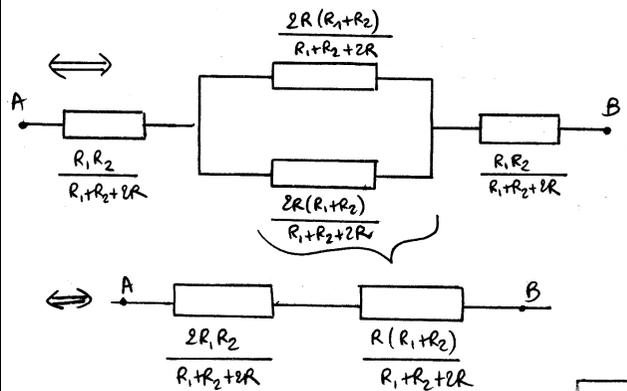
$R_{eq} = \frac{2R_1 R_2 + R R_1 + R R_2}{2R + R_1 + R_2}$
